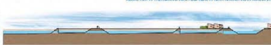
SECTION B-B: CONNECTION FROM SECONDARY CANAL TO STORAGE POND
